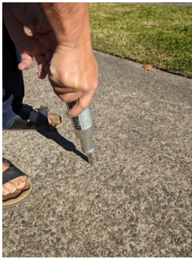
Testing concrete with the Hammer
