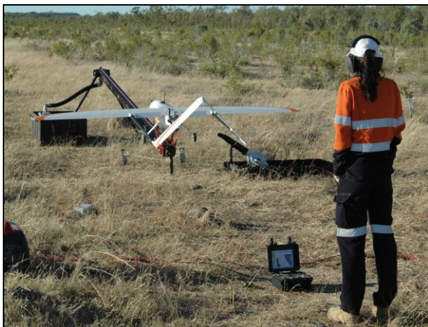
LiDaR Drone on launching ramp
