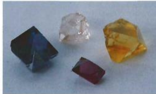
Figure A-1. Russian laboratories have produced flux-grown synthetic spinels in a variety of colors other than red and blue. These samples, reportedly grown on an experimental basis, range from 0.80 to 3.76 ct. Photo by Maha DeMaggio.
